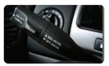
To turn the Cruise Control system on or off, press and release the ON-OFF-CANCEL switch located on the Turn Signal/Multifunction Lever. Cruise Enabled will be momentarily displayed in the Trip Computer window and the Cruise indicator will remain displayed while Cruise Control is enabled.
